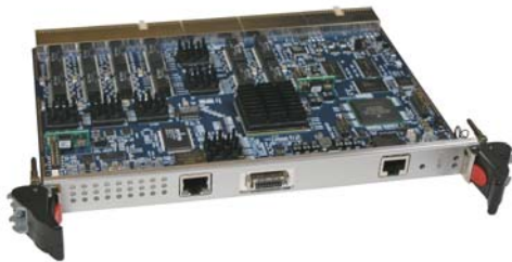
CSB4624 : DTI's CompactPCI Ethernet Switch
