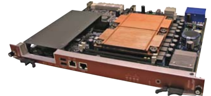
AdvancedTCA Node Board based on two AMD Opteron Socket F (1207) Processors
