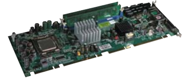
PICMG 1.3 Processor Board based on the Intel® Core 2 Duo™ 45nm LGA-775 package CPU
